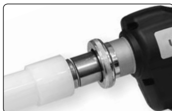
Figure 4-3: Slide Expander Head into Tubing
