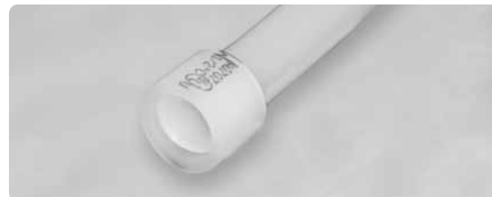
Figure 3-5: Place ProPEX Ring on Tubing
