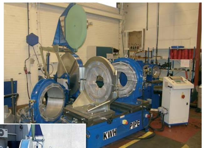
**PL 800 CNC** 400 V 3Ph. 50 Hz (standard) - 23 kW - 35 A
