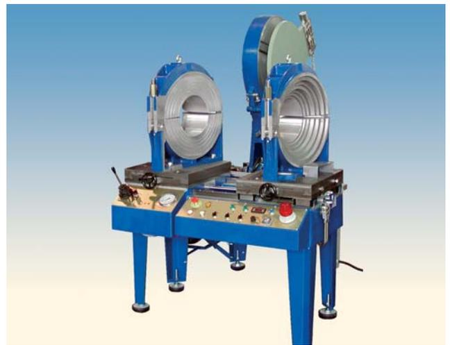
**PL 500 CNC** 400 V 3Ph. 50 Hz (standard) - 11 kW - 15 A
