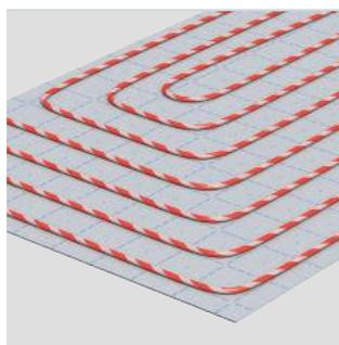
*Uponor Klett Twinboard Ideal for fastening the Uponor Klett pipes to any existing floor insulation materials. The 2.4 m<sup>2</sup> large foldable hollow-chamber boards do not require much storage space, are easy to transport thanks to their low weight of only 1.9 kg and are very easy to work on the building site.*
