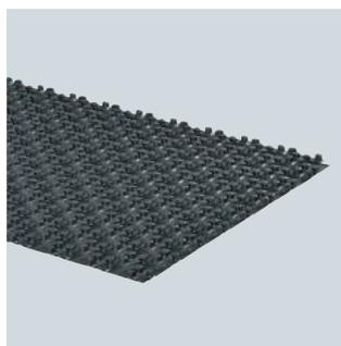
*Uponor Nubos nub foil – for laying on existing insulation. Foil element without back-foaming. Vacuum-formed PS deep-drawn foil made of high-impact polystyrene with integrate pipe holder nubs for reliable observance of the pipe spacings and for exact height fixation of the Uponor system pipes.*
