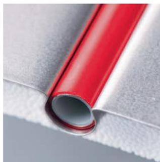
**The Uponor Siccus dry system can be used universally as an underfloor heating in a multitude of floor structures both in new buildings as well as in renovation work. In addition the system is optimally suitable for energy-related retrofit thanks to its low structure height and its low weight.**
