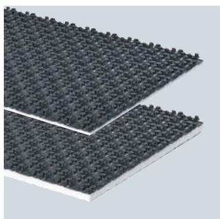
*Uponor Nubos nub panel for right-angled and diagonal pipe laying in different pipe spacings. Optimal adaptation to existing room geometries with minimal waste cut through two-sided overlapping edge studs. Type ND 30-2 for universal usage in residential and commercial buildings up to 5 kN/m<sup>2</sup> Type ND 11 for service loads up to 30 kN/m<sup>2</sup>.*
