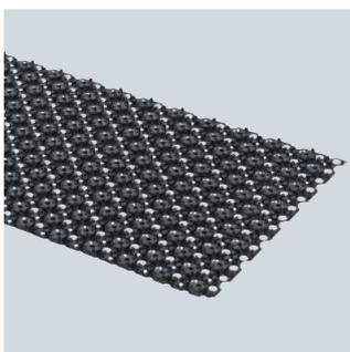
*Uponor Minitec foil element: stable and low pipe panel with integrated pipe guide for observance of laying spaces conforming to standard, for holding Uponor Minitec Comfort Pipe 9.9 mm pipes. Pipe laying straight and diagonal possible, with undercut, deep-drawn pipe retaining studs*
