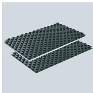
*Uponor Tecto nub panel with insulation ND 11 or ND 30-2 with impact sound insulation. Pipe holding sheet plate made of EPS and back-foamed covering foil. For Uponor system pipes 14 – 17 mm. Laying spacing 10/15/20/25/30 cm. Two-sided overlapping to ensure screed-proof connection.*
