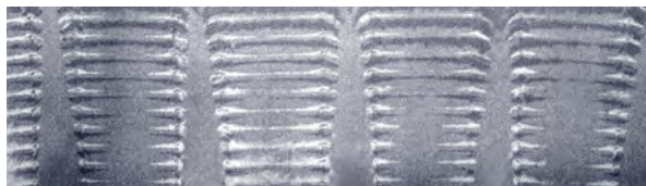
Figure 7-41: Expansion without proper rotation
