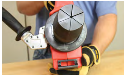
Figure 7-13: Correct expansion head alignment
