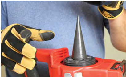
Figure 7-10: FORCE LOGIC expansion head installation
