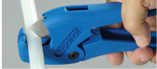
Figure 7-30: E6081128 pipe cutter (plastic)
