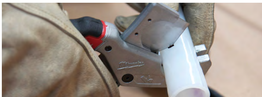
Figure 7-39: Cut pipe at marking
